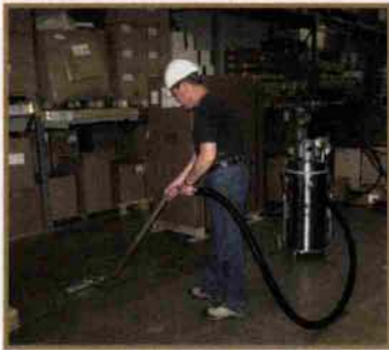
Figure 2: Powder coating facilities should develop and implement hazardous dust inspection, testing, housekeeping, and control procedures in order to prevent dust-related explosions.
